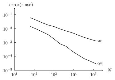
Fig. 2. Root mean squared error for estimating the first parameter of the pump model.
